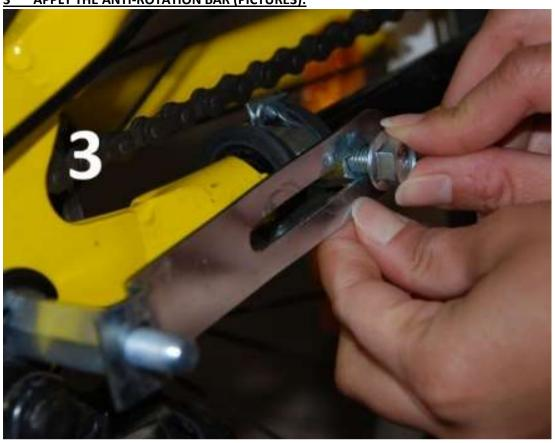
4 FIX THE BAR POSITIONING THE SUPPORT AND THE SCREW AT ITS END, WITHOUT TIGHTENING THE SCREW (PICTURE 4):
