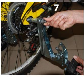
7 MAKE SURE THAT THE STWHEELS HAVE THE ADJUSTING PIN TO THE FIRST STAGE, SWINGING THE BIKE TO THE MINIMUM AS FROM (STEP (1) OF THE INSTRUCTIONS). POSITION THE BICYCLE PERPENDICULAR TO THE FLOOR. MAKE SURE THAT THE WHEEL OF THE BICYCLE AND THE WHEELS OF THE BALANCE DISPENSERS CORRECTLY GROUND TO EARTH AND TIGHTEN ALL THE SCREWS (PICTURES 8-9-10-11):
